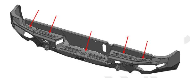
1. Carefully place the bumper up to the frame and fasten using the 7/16"-14 hardware. Adjust the bumper fitment and tighten all hardware.
