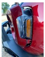
3. Now that the grill is free, disconnect your camera and camera washer spray line, above your passenger headlight. Once those items are disconnected, remove grill and set aside. Uninstall your camera from the grill and remove the factory camera harness and the sprayer tube. (Washer spray tubing will need to be capped or plugged: plug with a 1/4" bolt and zip tie)
