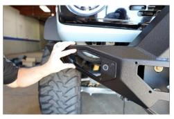
Note: Do not over tighten sensors. If you choose to unplug the sensors from the harness, and the sensors are not working properly after installation, use CRC Dielectric grease PN#05113 on all sensors and main harness plug.
