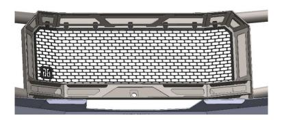
3. Install the mesh by sliding the top tabs under the webbing on the Extreme Guard. Once the tabs have are slid into place, bolt the mesh in place using the provided 1/4"-20 hardware. (If you have Adaptive Cruise Control, you will want to leave the two driver side bolt locations open.
