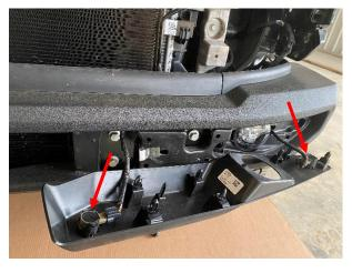
2. Once the plastic covers are removed, (a) locate the front sensor harness plug behind the driver side headlight and fender liner, (b) and unplug the harness. Now remove the 6 frame bolts using an 15mm socket, and the front bumper will come off.
