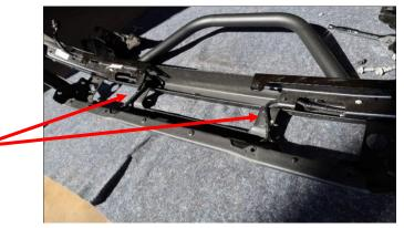
Once the bumper is off, locate the (6) bolts holding the skid plate, and remove the skid plate using the 15mm socket.
