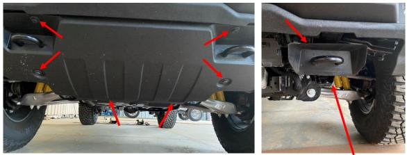
4. On the base model Bronco, the tow hooks may need to be cut out to complete installation.
