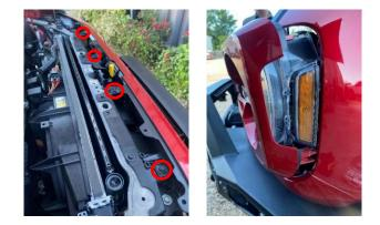
3. Now that the grill is free, disconnect your camera and camera washer spray line, above your passenger headlight. Once those items are disconnected, remove grill and set aside.
