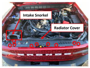
Once the radiator cover has been removed, remove the
