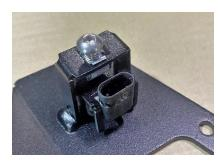
4. Install 1/4"-20 cage nuts into the fog light buckets. Next, install fog light pods onto the fog light buckets if applicable, then install the fog light buckets onto the bumper along with the sensor plate for the fog lights using 1/4"-20 x 3/4" hardware. Be sure to plug in the sensor to the harness before fastening to bumper.
