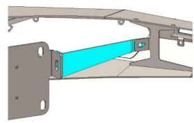
3. Run the factory harness through the bumper allowing for sensor plugs to position accordingly. Install the side markers at this time. Next, install 1/4"-20 cage nuts into the parking sensor plates and center mesh. (Images below are example sensor plates and center mesh). Then slip the sensor tab over the sensor, with the tabs fitting around the plug (Image
