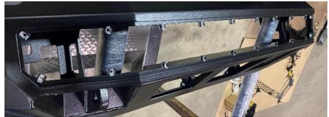
2. Carefully place the bumper up to the winch mount and fasten using 4x 7/16"-14 hardware. Next, fasten the wing brace from the winch mount to the bumper, as shown below using 2x 7/16"-14 and 2x 5/16"-18. Adjust fitment vertically and horizontally, then tighten all hardware.
