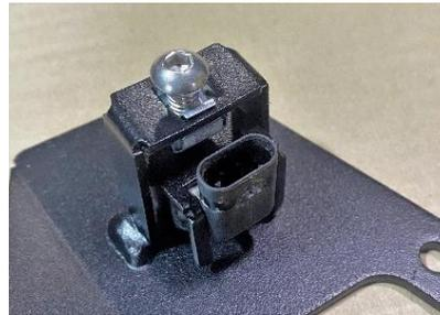
4. Install 1/4"-20 cage nuts into the fog light buckets. Next, install fog light pods onto the fog light buckets if applicable, then install the fog light buckets onto the bumper along with the sensor plate for the fog lights using 1/4"-20 x 3/4" hardware. Be sure to plug in the sensor to the harness before fastening to bumper.
