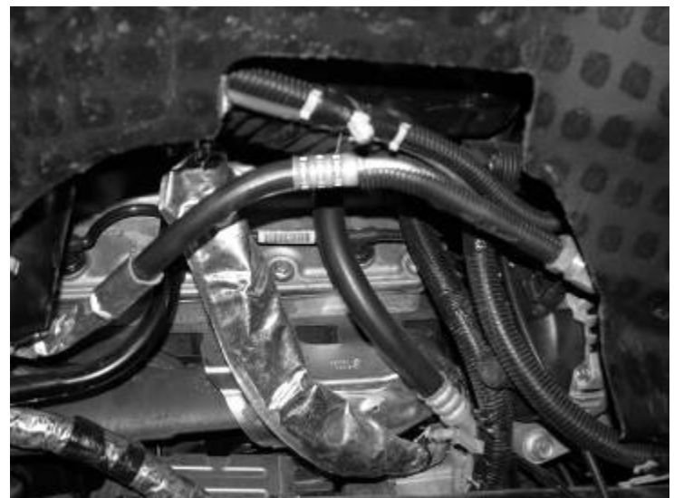
Photo shows bent A/C line
