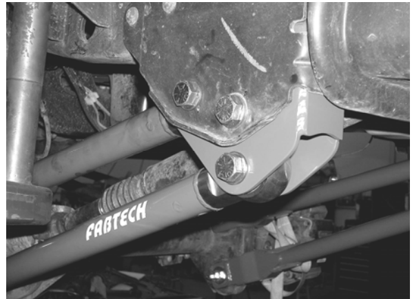
Assembly of the FT292 Alignment Cam
