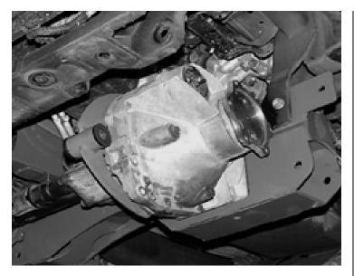
25. Attach the Fabtech front crossmember into the lower control arm pockets using the stock hardware. Leave loose. SEE PHOTO BELOW.
