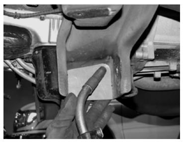
18. Locate the mounting bushing eye on the upper front side of the differential housing and mark the housing with a cut line flush to the housing. Using a sawzall cut the entire ear off the housing. Take care not to cut into the flat portion of the housing. SEE PHOTOS BELOW.
