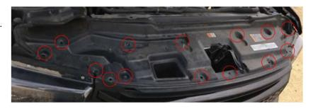
2. Remove the (8) 10mm bolts and remove the grill by pulling outward on it.
