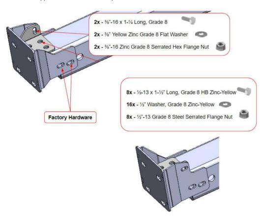
1. Attach the bumper with the 1/2" stainless hardware, leaving enough space to adjust the bumper as needed into position. Using a tape measure, adjust the bumper vertically and horizontally to the desired body gaps. Once the bumper is lined up, tighten all hardware for the bumper and the mounts. Using jack stands or an additional person to help support the bumper is recommended.
