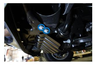
11. Remove 18mm bolt and 15mm bolt (will require extension to reach) from bumper mount (each side)
