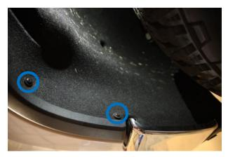
2. Remove fender flare and remove one 7mm bolt
