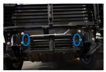
15. Remove 15mm bolts to uninstall factory bumper mounts. (Reinstall grille, all trim panels)
