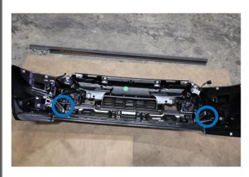
12. Pull back bumper to remove block heater plug (if equipped), park sensors/fog lights cables (if equipped), then remove the bumper.
