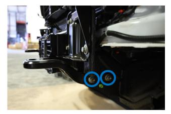
14. Remove top four 7mm bolts securing the active aero shutters which will hang, connected until bumper installation.
