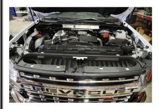
6. Remove T25 screws from hood latch, and remove hood latch
