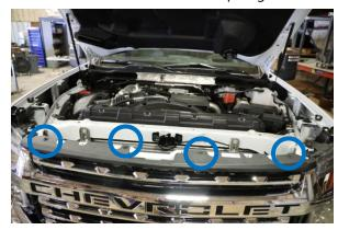
9. Remove grille and detach front camera cable (if equipped). You will remove the camera at this time and connect the <u>camera cable extender (sold separately)</u>.
