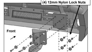
(Fig 9) Attach passenger/right side of Bumper to Frame Bracket
