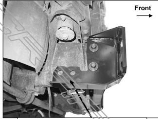
(Fig 6) Mounting holes not used for this particular installation (arrow).
