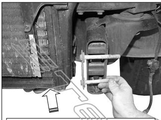
(Fig 3) On diesel models only: Leosen and lift intercooler up to remove double bolt plates
