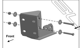
(Fig 5) Attach passenger/right side Frame Bracket to outside of frame
