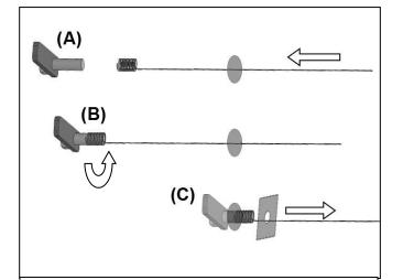
(Fig 4) On models with reinforced cross member, insert coiled end of Fish Wire through hole in front of cross member (A).
