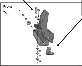
(Fig 5) Attach Support Bracket to Frame Bracket and Bolt Plate in cross member
