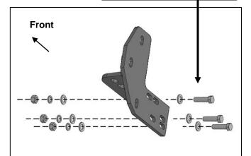
(Fig 2) Attach driver/left Frame Bracket to inside of end of frame. Line up correct slots in Bracket with mounting holes for factory bumper bracket
