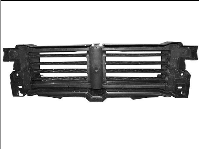
(Fig 18) Remove inner shutter assembly from plastic outer housing (if equipped)
