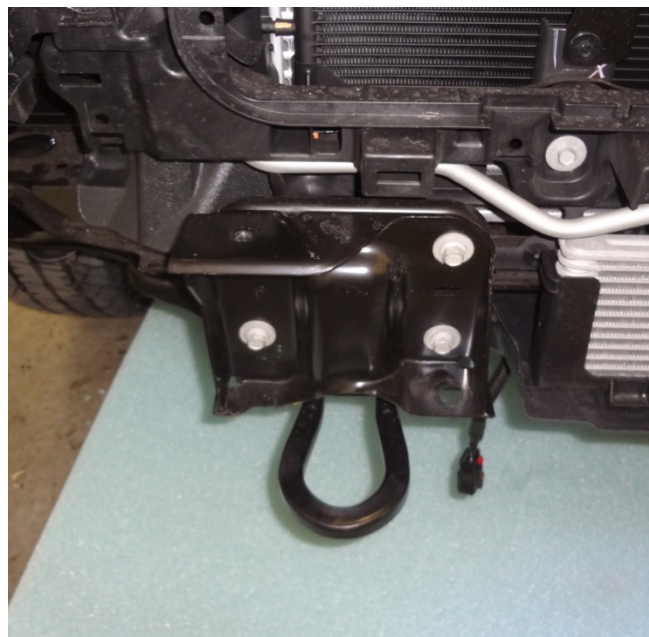
Figure 3b (TOW HOOK & OEM MOUNTING BRACKET)
