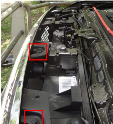
Figure 2a-bolts on LH side
