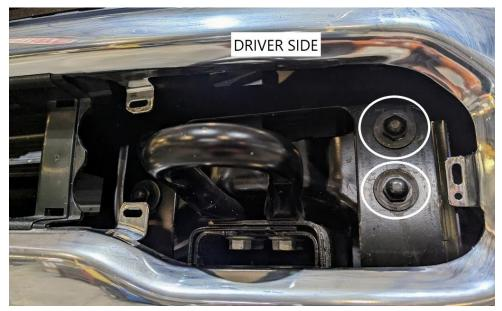
4. To install the bottom bracket, remove the two 18mm nuts from the side of the frame. Install the bottom mounting brackets. Line the top hole of the bracket over the top hole of the bumper. Reuse factory hardware.
