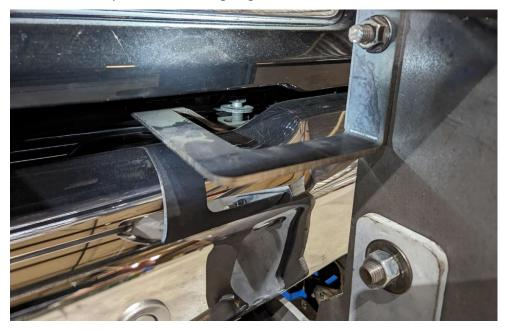
16. If the vehicle does not have a camera, install small insert by using the black button head bolts and nuts.
