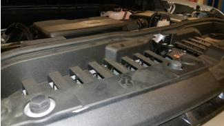
5. If vehicle is installed with a front camera, unhook the connector. The grille can then be removed by remove four 10mm bolts on top and four 10mm (two on each side) from the sides.
