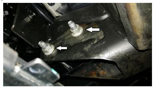
2. Install the bottom brackets by sliding the brackets from the back. The bracket mounts to the outer side of the frame. Reinsert the tow hook and use the 5" x ½" bolts to install. If no tow hooks use 1 ½" x ½" bolts. You may have to trim the plastic where the brackets come through the tow hook opening. NOTE: YOU MAY HAVE TO TRIM SOME OF THE PASTIC AROUND THE TOW HOOK AREA.
