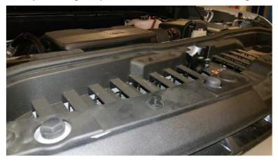
Remove the factory grille by removing the four 10mm screws on top and pulling on the grill clips.
