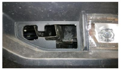
5. Slide the 5" tab w/the bolts through the top holes of the frame.
