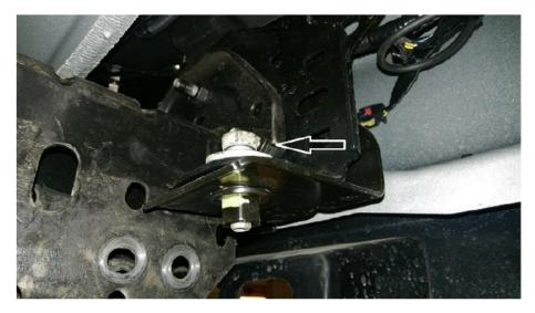
2. (*Diesel*) On the driver side, cut the front tow hook bolt off. You will use a ½" x 4" bolt to reinstall the tow hook later.
