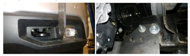
7. Reinstall the tow hooks. Use the factory tow hooks. If there are no tow hooks present, use  $\frac{1}{2}$ " bolts. Also, at this time tighten the 18mm bolt that was loosened in step 1.
