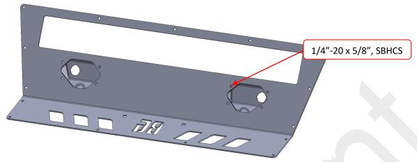
5. Install the sensor pod to the skid plate using 8x 1/4"-20 x 5/8", SBHCS
