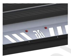
6. Install 2x 1/4-20 Cage Nut into square holes on each side of BG logo
