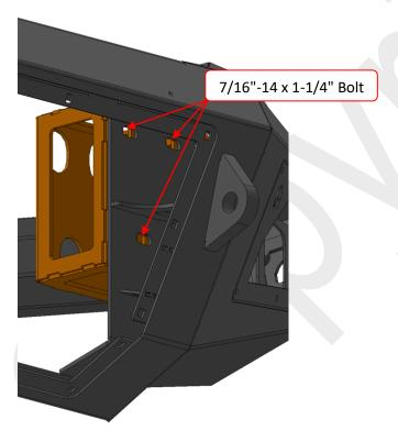
1. Install **3x 7/16"-14 x 1-1/4" Bolt** securing the bumper to each mount.
