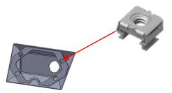
4. Install **4x 1/4-20 Cage Nut** to each sensor pod. This will only apply if your truck has factory front sensors
