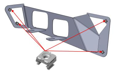
1. Install 4x 1/4-20 Cage Nut onto each fog light bucket.
