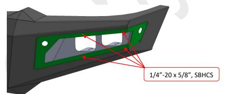
3. Finally install 4x 1/4"-20 x 5/8", SBHCS with 4x 1/4-20 Serrated Flange Nut.
