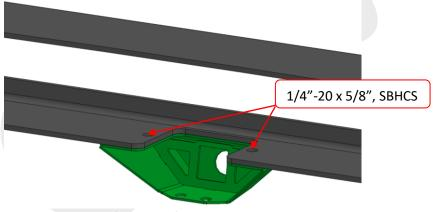
2. Install 2x 1/4"-20 x 5/8", SBHCS securing the camera pod to the sport bar.
