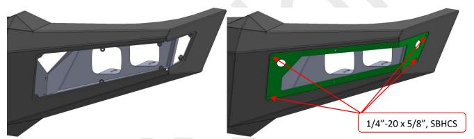
2. Next insert the fog light bucket into the bumper and secure using 4x 1/4"-20 x 5/8", SBHCS.
