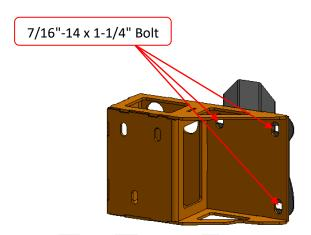
1. Install **3x 7/16"-14 x 1-1/4" Bolt** securing each mount to the frame.
