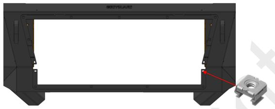
1. Install **15x 1/4-20 Cage Nut** to the skid plate trim ring.
