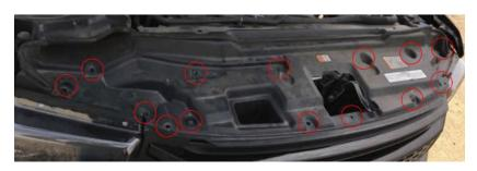
2. Remove the (8) 10mm bolts and remove the grill by pulling outward on it.
