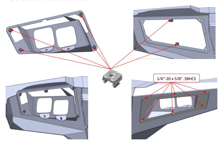
Next insert the fog light bucket into the bumper and secure using  $6x \frac{1}{4}$ "- $20 x \frac{5}{8}$ ", SBHCS
