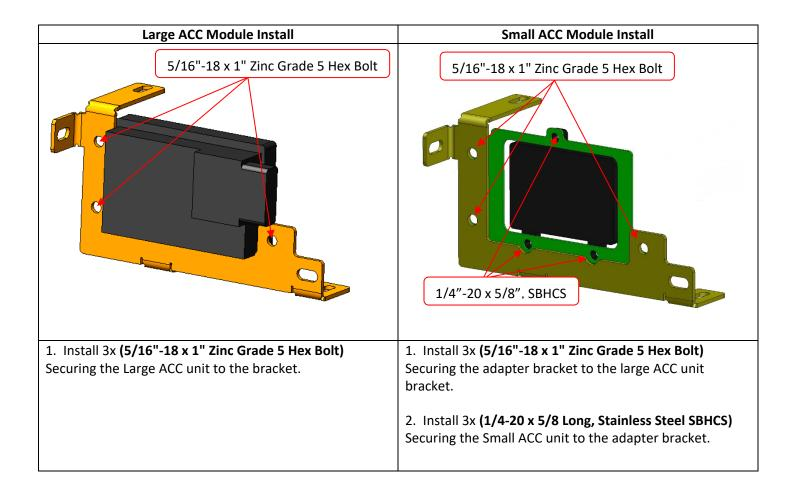
Note: Some slots on this bracket will not be used for this install. This is a universal ACC bracket used on several different models.
