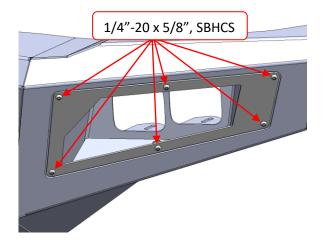
Next insert the fog light bucket into the bumper and secure using 6x 1/4"-20 x 5/8", SBHCS
