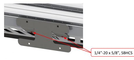
2. Then install license plate bracket to skid plate using two 1/4"-20 x 5/8" button head screws
