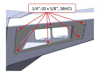
Next insert the fog light bucket into the bumper and secure using 6x 1/4"-20 x 5/8", SBHC
