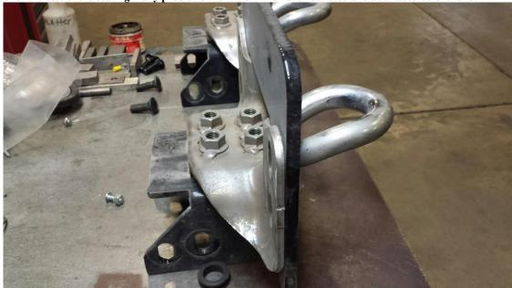
9. On trucks that have the extra towing package cooler, you will need to flatten or cut off the two tabs that hook under the frame rail. *See photo below*
