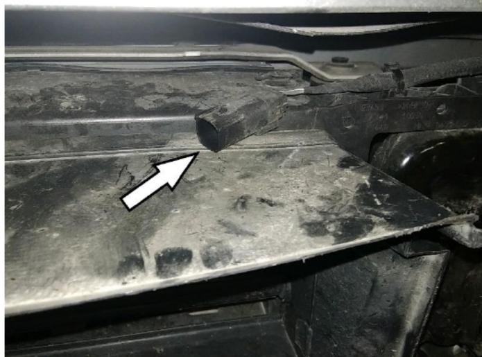
3. If tow hooks are present, remove them. Mount the bottom brackets along with the tow hooks to the bottom of the frame. Mount the top brackets to the two outside holes in the frame plate. Use 1/2" hardware provided. Brackets should be about 39 1/2" O.D. apart. (Hand tighten)
