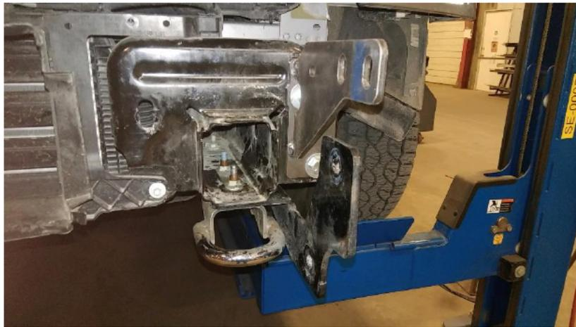
4. Remove the wiring harness from the factory bumper. Also remove fog lights and adaptive cruise if present.
