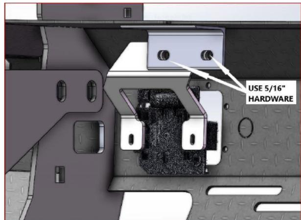
8. Install the center inserts by using the black button head bolts, nuts, and rubber washers. **NOTE: IF THE ADAPTIVE CRUISE DOES NOT FUNCTION PROPERLY, REMOVE THE INSERT FROM IN FRONT OF THE MODULE AND RETEST.**
