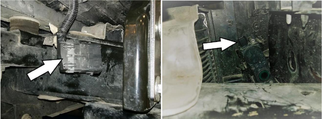
2. To remove the factory bumper, you will need to remove the six 21mm mounting nuts (three on each frame horn). There will be one more connector above the bottom louver system on the driver side. Carefully pull the bumper away from the frame then unplug connector.
