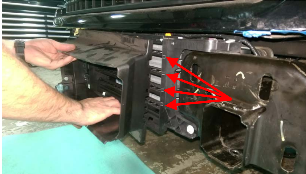
Figure 4a (Removing shroud from louvers)
