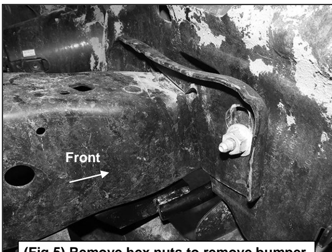
(Fig 5) Remove hex nuts to remove bumper
