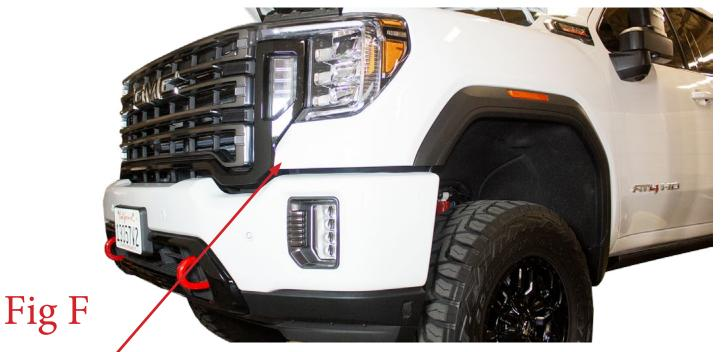
Release the clips along this side of the valance, but do not pull the valance all the way off the vehicle.
