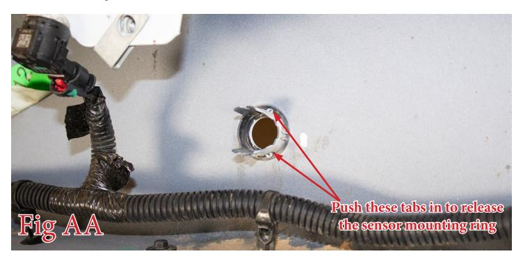
29. Release the series of clips holding the harness to the bumper. Then remove the parking sensor/fog light harness from the bumper. (Fig AB) Make sure to keep track of the position this was mounted on the OEM bumper so it can be mounted on your new bumper in the same position.
