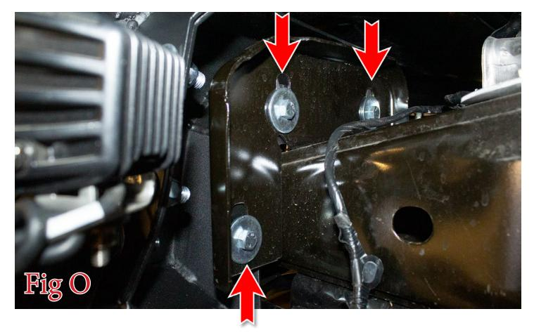
21. Align your bumper so it is centered left to right and straight in relation to the grille/valance. Then, tighten the 3/8" mounting bolts to 25 foot pounds.
