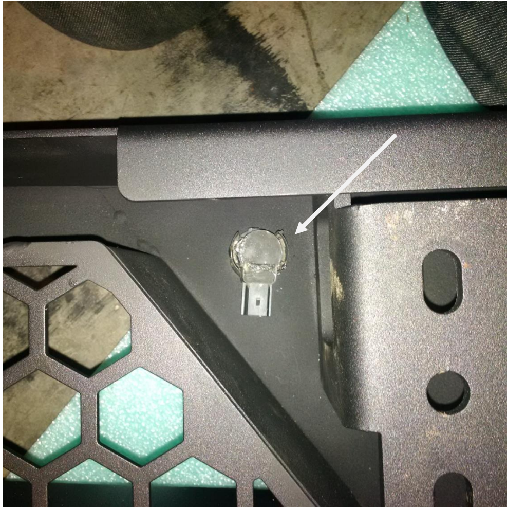
Figure 4 Outer passenger side sensor orientation
