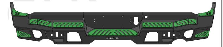
1. Install all step pads using 36x 1/4-20 x 5/8 Long bolt
