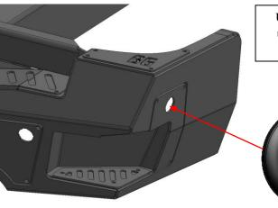
Use provided sensor plugs for any unused sensor holes. Some trucks come with 4 sensors instead of 6.
