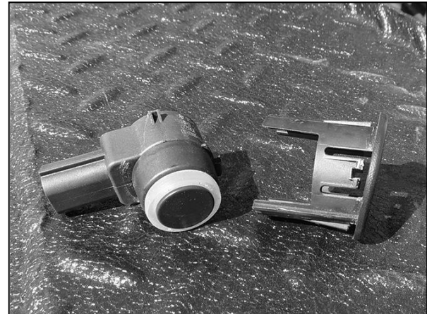
(Fig 9) Remove the seal from the end of the sensor. Install larger Foam Washer (Fig 10)
