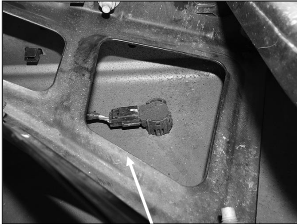
(Fig 8) Unplug the sensor first then remove the sensor from the mounting sleeve
