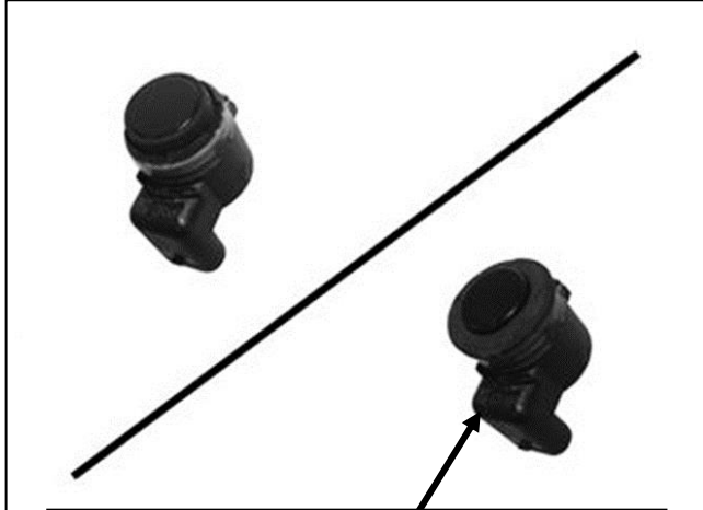
(Fig 6) Remove silicone seal from sensor. Slide Foam Washer over end of sensor
