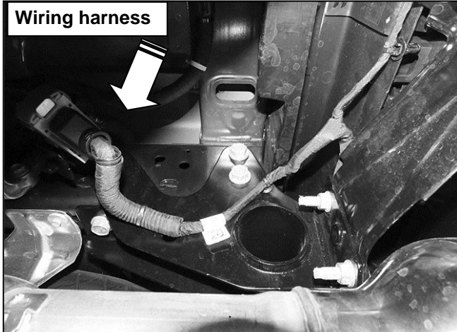
(Fig 1) Unplug wiring harness leading to bumper
