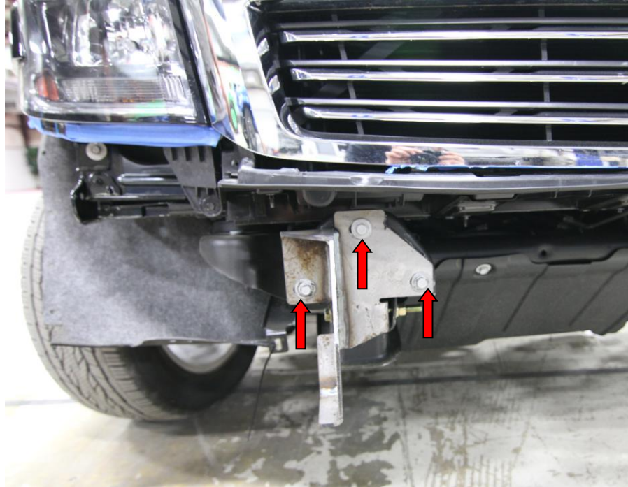
Figure 6 – INTERMEDIATE BRACKET INSTALLATION – TOP VIEW
