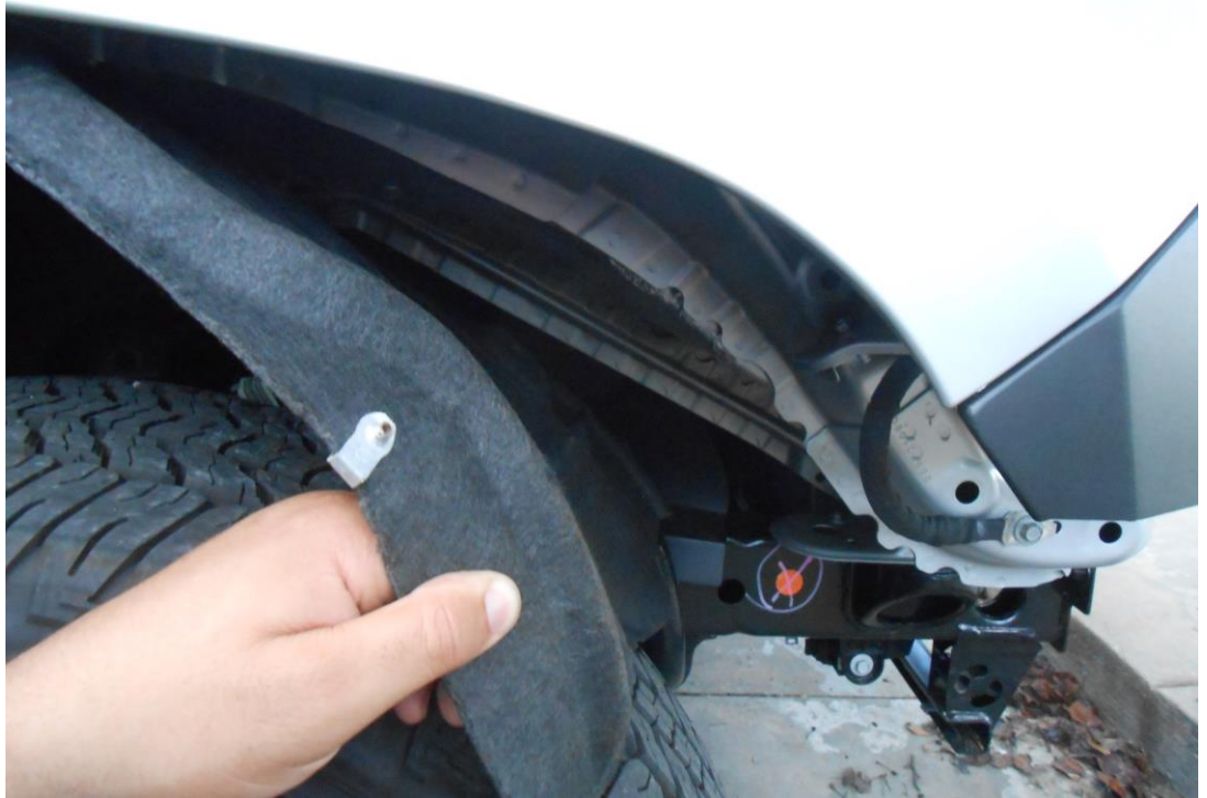
Figure 6a (wheel well liner pull back)
