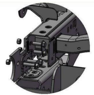
7. (2023 models) Remove the bumper bracket by removing the two 21mm bolts and two 15mm bolts from each side. Also, remove the one 24mm (15/16") bolt from top of the frame.
