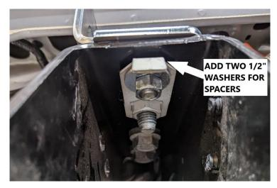
10. Set up one of the bolt tabs inside the frame so it is inline with the holes of the frame. May need to prop it up with a block. Makes it easier to install.
