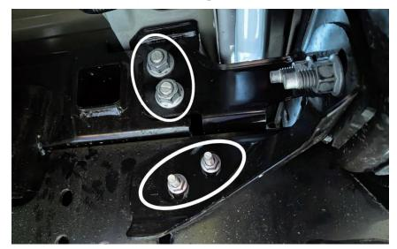
8. (2017-22) Install the Ranch Hand bumper. Reuse the factory 21mm nuts and bolts to mount.
