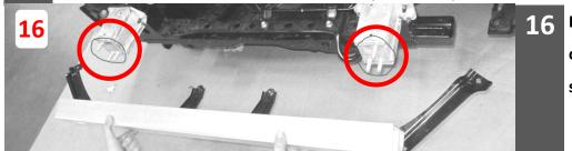
Remove the six 14mm nuts on the stock bumper with a socket.
