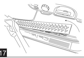
Pull wires from grommet and route back along factory wire harness to back door sill plate.
