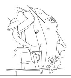
Mount controller with the two 11" tie wraps to factory conduit. Route wire harness under core support and down toward controller. Attach harness to controller (make sure connector locking tabs fully engage).
