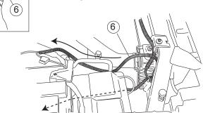
Route longer leg of harness across front and down under driver side. Secure harness with tie wraps and reinstall shroud.
