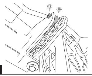
Slide mounting T-nut into position, Center board in rail pocket. Tighten fasteners to 10 ft-lbs.
