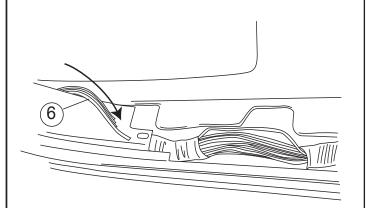
Locate the appropriate signal wires as noted below. Note: There may be up to five Black with Blue Stripe wires; use the one that looks unique (ie. different blue stripe... weight and shade).
