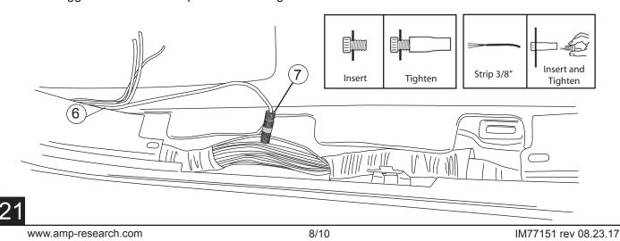
Connect harness to motor. Secure harness with tie wraps.
