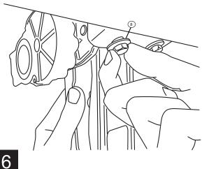
Install provided spacer (19) and M6 bolt (12) into upper mount as shown on both the Drive and Idler linkages. Do not tighten.
