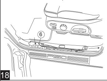
Remove rear door step plate and open wire bundle. Route trigger wires to rear door sill plate.
