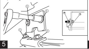
Thread supplied bolts 2x (8) into Front Idler Linkage. Repeat step for Rear Drive Linkage. Do not tighten.
