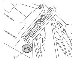
Attach motor to harness. Using a 4mm hex Torque to 36 in-Lbs.
