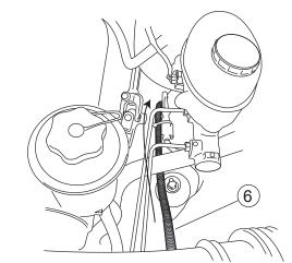
Puncture grommet and thread all four trigger wires up into the cabin of vehicle. The grommet is located on driver-side behind forward linkage assembly.
