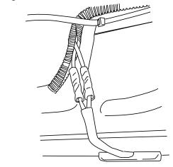
Close and wrap conduit with electrical tape. Secure all loose wires with cable ties. Pull lamp wires upward to avoid any wire snagging.
