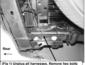
(Fig 1) Unplug all harnesses. Remove hex bolts from bottom of bumper reinforcement (pictured) or receiver hitch to remove bumper assembly **WARNING!** Do not crawl under bumper unless the bumper is properly supported on blocks or stands or the bumper may fall.
