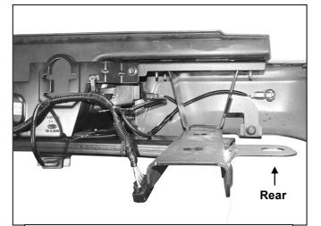
(Fig 3) Disassemble bumper to remove bumper reinforcement (pictured) or receiver hitch, wiring harness, sensors, license plate lights and trailer plug as equipped
