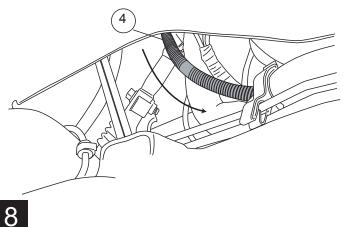
Poke hole through rubber grommet near front door on underside of floor panel with small phillips screwdriver. Push both wires through hole. (See Step 11 for passenger side notes.)
