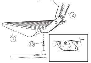
Tighten button head fasteners and M8 nuts on driving and idler linkages to 16 ft-lbs.
