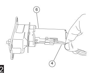
Slide rubber grommet on wire harness into slot of motor cover. Insert motor cover onto motor.
