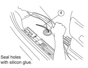
Locate wire loom in door sill. Carefully remove wire wrap and find the trigger wire.
