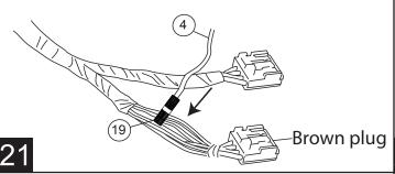
Insert plug from wire harness onto motor.
