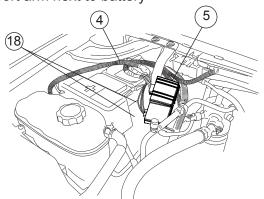
Plug in wire harness. (Ensure that locking tabs engage.)
