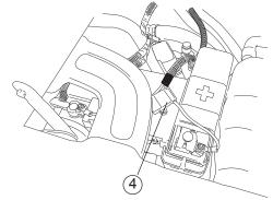
Attach ground lead to negative battery pole.
