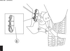
Using the two 11" cable ties, mount controller to support arm next to battery
