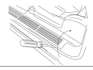
Pull up the carpet and thread both wires through the floor panel (same steps on passenger side EXCEPT drill 9/32" hole in metal and add rubber grommet).
