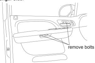
Remove door latch cable from door panel. **Repeat on passenger side.**
