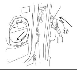
Feed longer wire of Step 11 through tube into door and pull out plastic tube on door side. Route wire along harness to switchplate.
