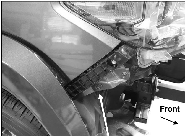
(Fig 3) Remove plastic block (arrow) from front edge of fender. Reinstall hardware to secure headlight
