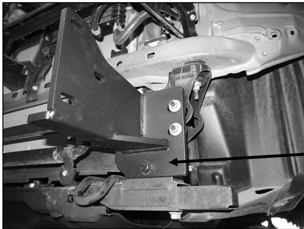
(Fig 8) Driver/left Mounting Bracket attached to end of frame
