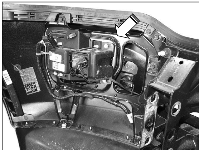
(Fig 11) Remove the wiring harness, sensors and fog light assemblies from bumper (if equipped)
