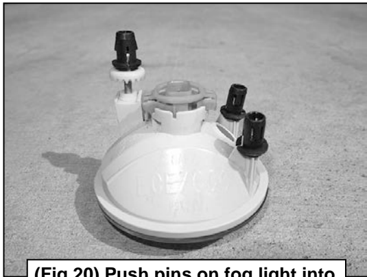
(Fig 20) Push pins on fog light into mounting tabs (if equipped)
