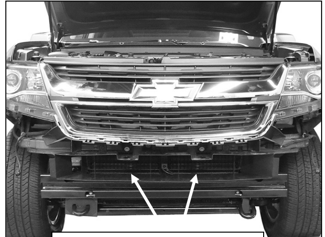
(Fig 7) Remove (2) hex bolts (arrows) to remove air deflector
