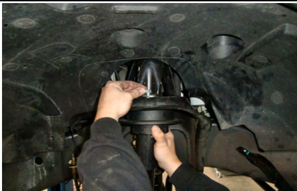
Attach ReadyLIFT Coil Spacer with supplied nuts "Leave Loose"
