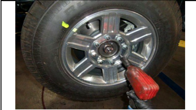
Raise front end of vehicle, support frame and remove wheels
