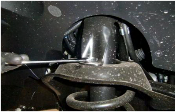
Loosen upper shock tower. Leave tower and nuts on.
