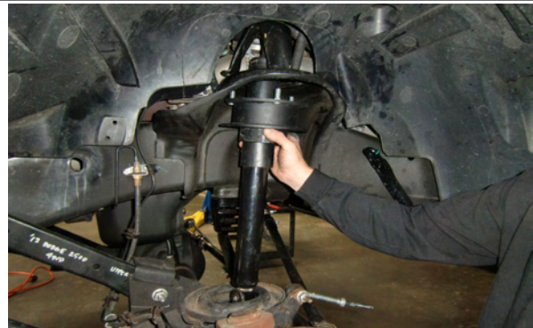
Install ReadyLIFT Coil Spacer
