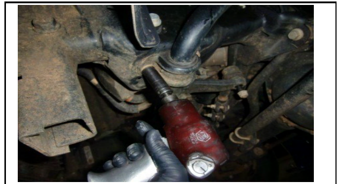
Disconnect sway bar from frame.
