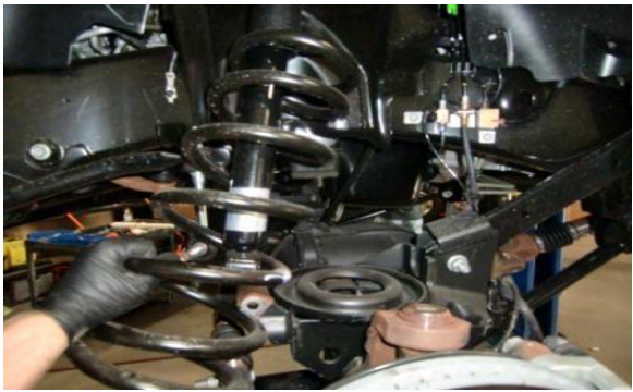
Remove spring towards the front of vehicle.
