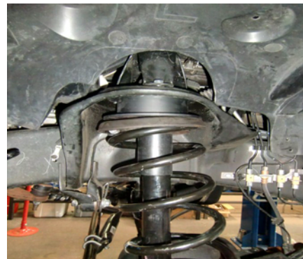
Re install Isolator and coil spring
