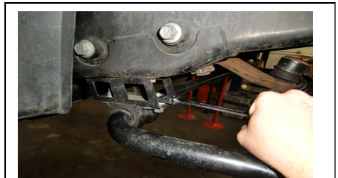
Tighten drop down bracket and sway bar.
