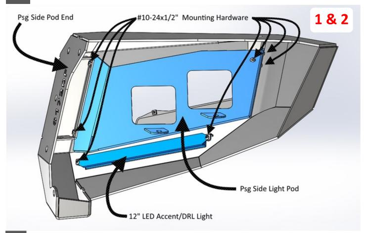
Align and install each kit pod end using Qty:  $6 - 7/16"x 1 \frac{1}{2}"$  bolts, nuts, lock washers and washers.
