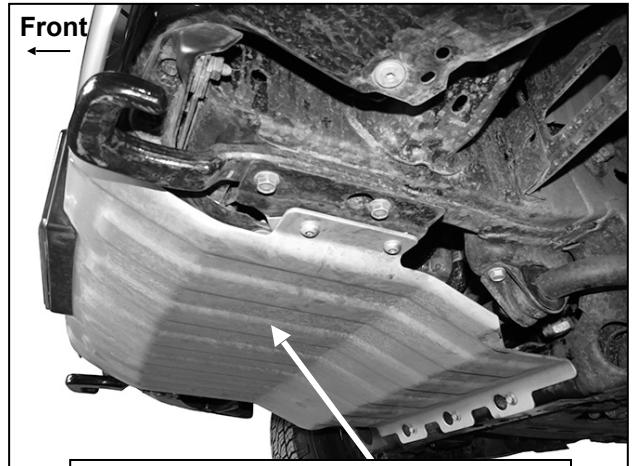
(Fig 4) Remove skid plate if equipped
