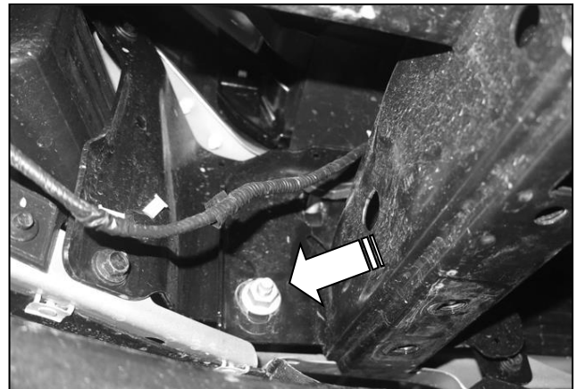
(Fig 2) Remove factory hex nut (arrow) from back of bumper bracket (Driver side pictured)
