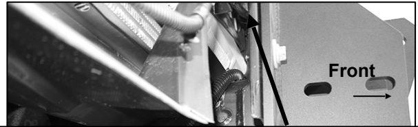
(Fig 19) Right facing Support Bracket installed
