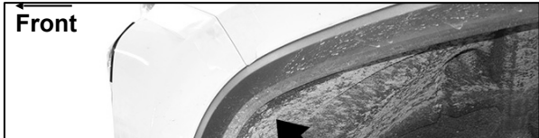
(Fig 1) Release hardware attaching fender liner from plastic panel (fascia-see arrows)
