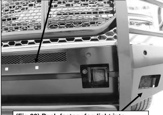
(Fig 20) Push factory fog light into mounting tabs (driver/left side pictured)
