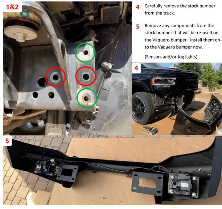
Note: Be gentle removing parking sensors. These are easily damaged if subjected to a sudden impact. To remove the sensors, from the rear use a pick tool and slightly pry the housing away from the tabs on the sensor. Push on the front of the sensor and it will slide out the back.
